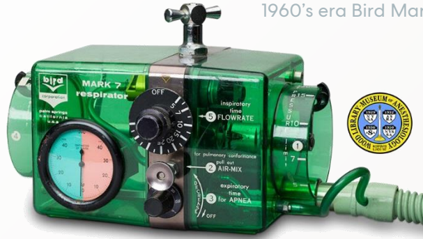
1960's era Bird Mark Ventilator
